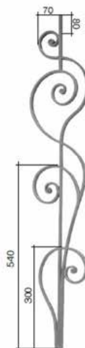
Art. 313A08 □ 14 x 8 mm H 1000 mm L 190 mm
